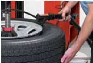
Blast inflation directs large blast of air for tough bead seating.
